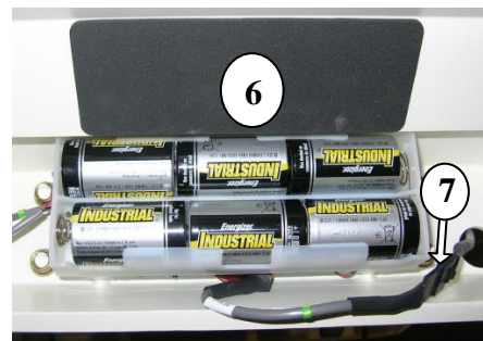
Figure 2: Display Cable Connector and Battery Compartment Cover
