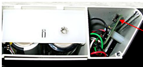
Figure 6: Display Board Calibration Switch Location
