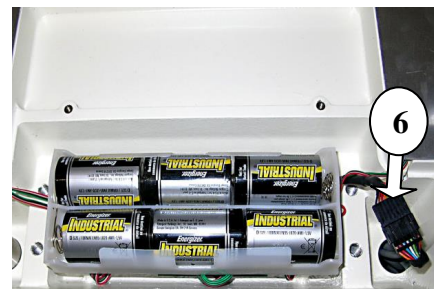
Figure 2: Display Cable Connector and Battery Compartment
